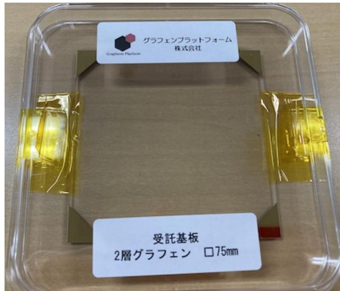
**Figure 2.11:** The graphene plate, which was fabricated by transcription of two 75 × 75 mm graphene sheets to 85 × 85 mm  $t = 2.0$  fused silica plate.
